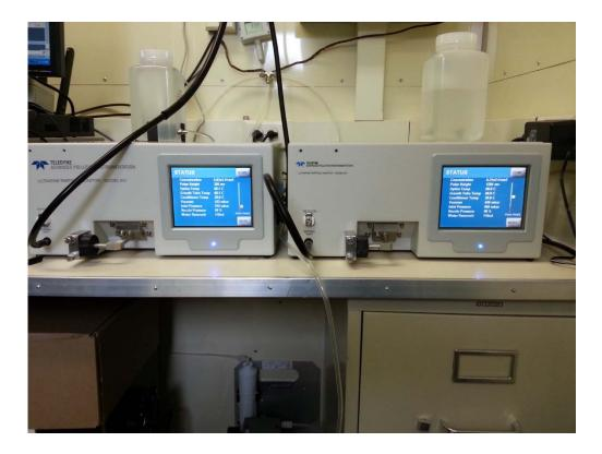
UFP range (0.001-0.1 Microns) API Model 651, TSI 3783 Water CPC Lower size cut 7nm (0.007 microns) 1 Micron Cyclone Inlet 2<sup>nd</sup> Unit is on Loan from the Manufacturer
