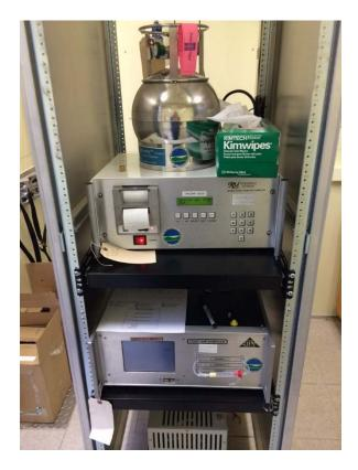
Computer controlled Canister Sampler
