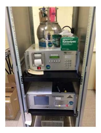
Computer controlled Canister Sampler
