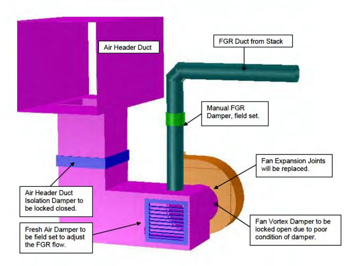
For Units #2/3 and #5/6, the FGR will be induced by placing the FGR duct right to the inlet of the FD fan (see pictures at end of quote).
