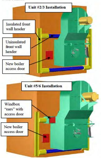
Units #2/3 and Units #5/6 have dual Todd burners with shallow windboxes. Coen proposes to replace these dual burners with single burner packaged units with all new fuel piping and windboxes. Switching from dual to single burners will reduce maintenance costs and improve reliability. The new, single burner windboxes will still be shallow enough to remove the oil gun without hitting the panel or wall.
