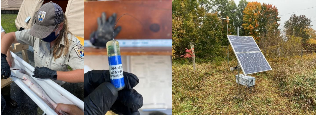
Figure 3. Radio tagging Atlantic salmon (left image), Sigma Eight Inc. radio telemetry transmitter (center image), and Sigma Eight Inc. radio telemetry receiver in the Winooski River.
