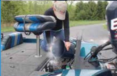
**DISINFECT** the boat's bilge area, all water-holding compartments, and other equipment with hot water at least 140°F or steam for at least 30 seconds before launching into another water body.
