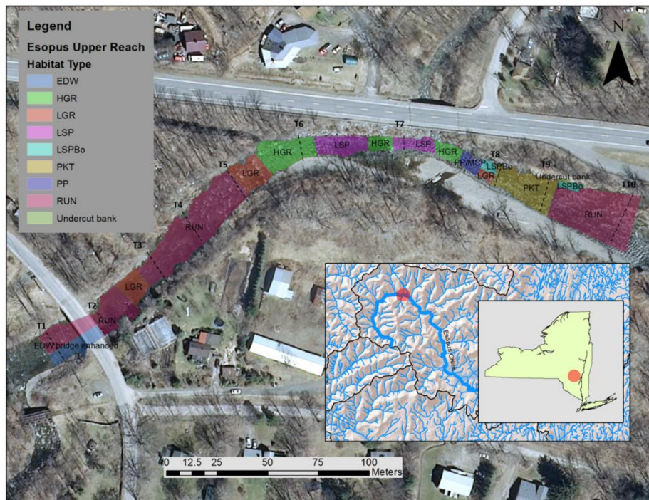
Figure 3. Example of a single reach scale mesohabitat map incorporating data on channel geomorphic habitat unit type, discharge, substrate, embeddedness, depth, instream and overhead cover, water chemistry data, temperature, land use, and riparian vegetation.
