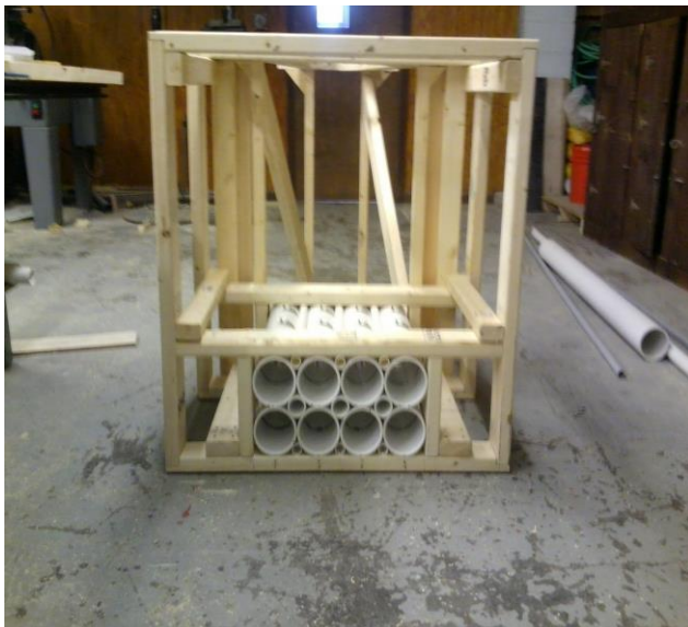
Figure 10. Top: Front view of the counter head that consists of eight four inch PVC tubes fitted with three stainless steel clamps, acting as sensors that measure water conductivity. Bottom left: View of fish counter head during construction. Bottom right: View of in-stream weir and fish counter.
