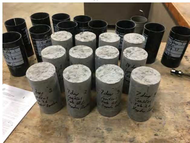
Figure 13. Cement made with pulverized glass at the World Center for Concrete Technology. Credit: Frank Roethel
