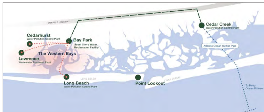
Figure 4. The Bay Park Conveyance Project: The project is rerouting the South Shore Water Reclamation Facility effluent from its current outfall in the Western Bays to connect to the existing Cedar Creek Ocean Outfall located three miles offshore in the Atlantic Ocean. The figure depicts the new conveyance pipeline under construction. Credit: Western Bays Constructors
