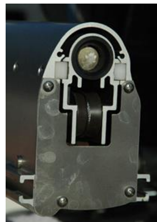
Example: A Minn Kota Talon power pole base can be prone to trapping sediment or vegetation
