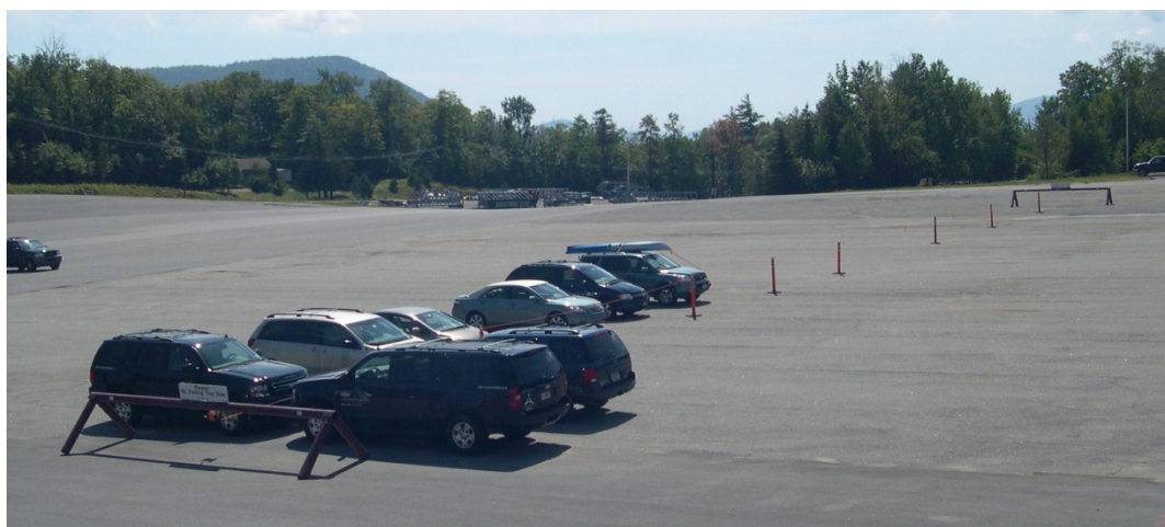
Photograph 10 - Parking lot using pipe sawhorses and plastic balusters to establish row locations
