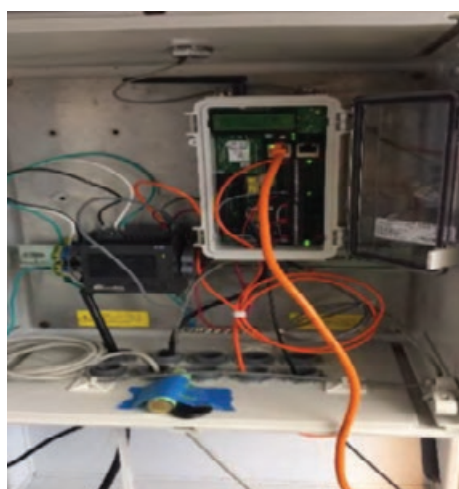
Figure 3: A fluridone injection unit (left), unit control dashboard (center), and cellular control device (right); credit: SePRO
