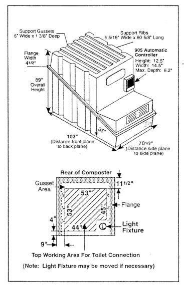
systems are 115VAC. The 905 displays information through an LCD panel and provides maintenance alerts through an audible alarm.
