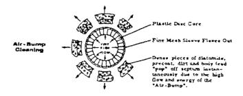
Instead of ordinary backwashing, which is often ineffective, Separmatic filters use the "AIR-BUMP" principle. Air, trapped in the filter dome, is released suddenly to provide a high energy, reverse flow through the filter. This action effectively pops off the dirty filter cake. During cleaning, the "AIR-VAC" system allows air to enter the tank, producing a vigorous scrubbing action on the surface of each filter element.
