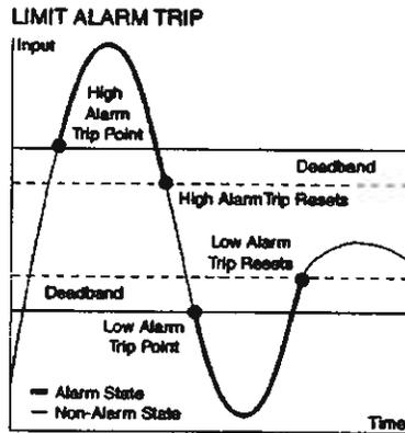
Figure 5. The SPA<sup>2</sup> can be used as a simple on/off controller such as those required in level applications (pump/valve control) when filling or emptying a container or tank.
