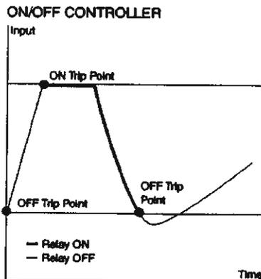
Figure 6. The SPA<sup>2</sup> can be set to trip when the input rate-of-change exceeds a user-selected rate (Delta) over a user-selected time period (Delta Time).
