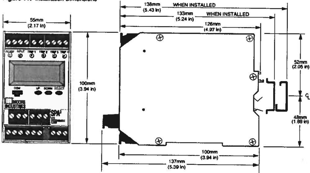
NOTE: While all SPA<sup>2</sup> models (model with HLPARG Input shown) are dimensionally identical, the SPA<sup>2</sup> that accepts temperature inputs (TPRG Input) features metal terminal blocks for enhanced reference junction compensation.
