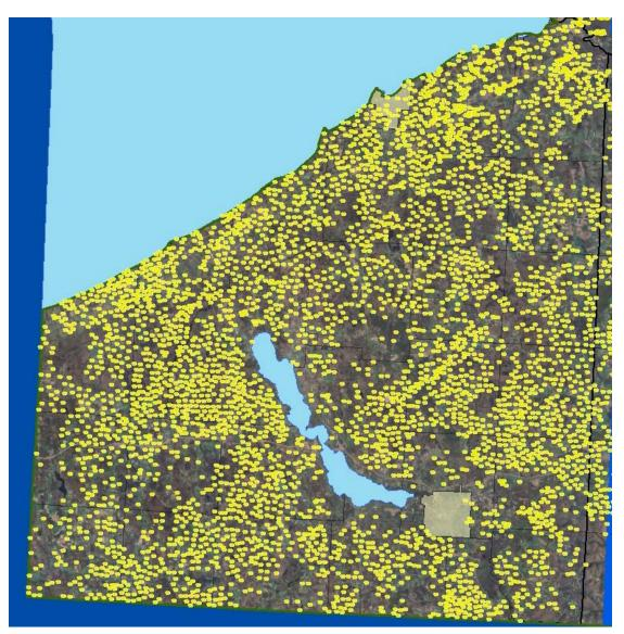
Photo 5.8 This map shows the locations of over 4,400 Medina formation natural gas wells in Chautauqua County from the Mineral Resources database. The wells were typically drilled on 40 to 80 acre well spacing, making the distance between wells at least 1/4 mile.
