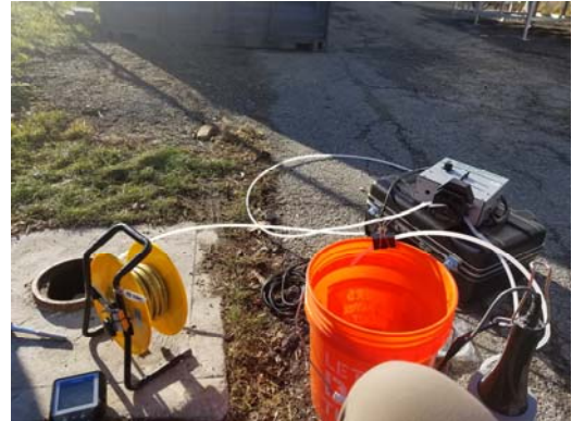
Photo 2.5: Typical groundwater sampling setup.
