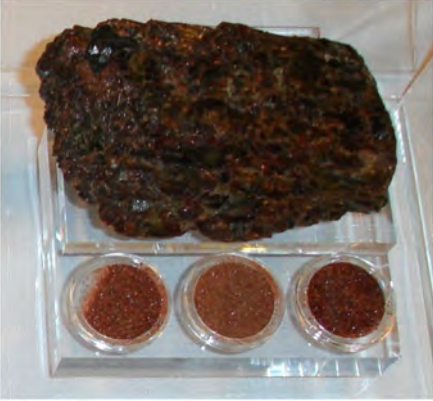
Closer view of a large garnet and some of the processed grade sizes for use in abrasives.
