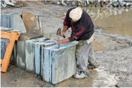
Using a hand chisel to split the rock into landscaping and building material.
