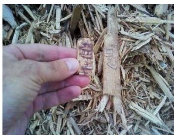
Figure 5 Rough grind mulch contaminated with colored plywood
