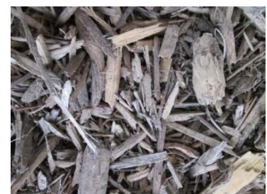
Figure 6 Finished mulch with CCA wood (note how difficult it is to see contamination once mulch is processed)
