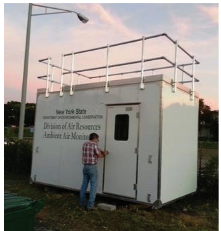
Example of a fixed air monitoring shelter which will monitor and record levels of particulate matter, gaseous chemicals, and track wind direction and speed.
