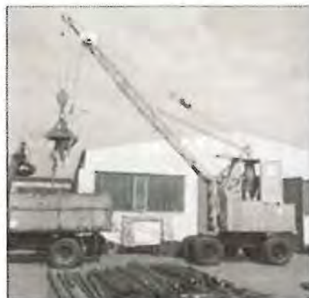
1962: Rope-driven S833 with elevated operator cab
