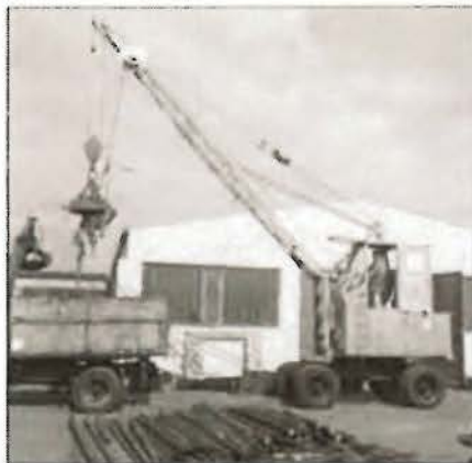
1962: Rope-driven S833 with elevated operator cab
