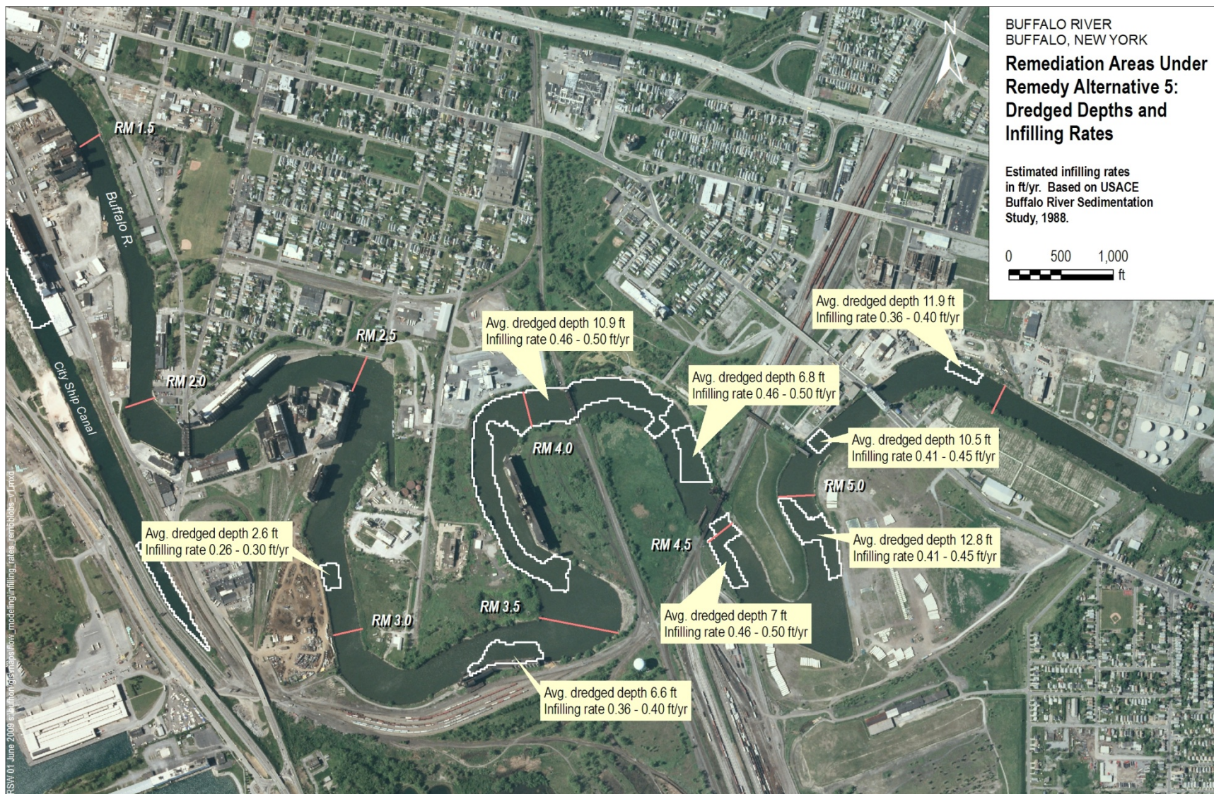
Figure 2: Remedy 5 Dredged Depths and Estimated Infilling Rates
