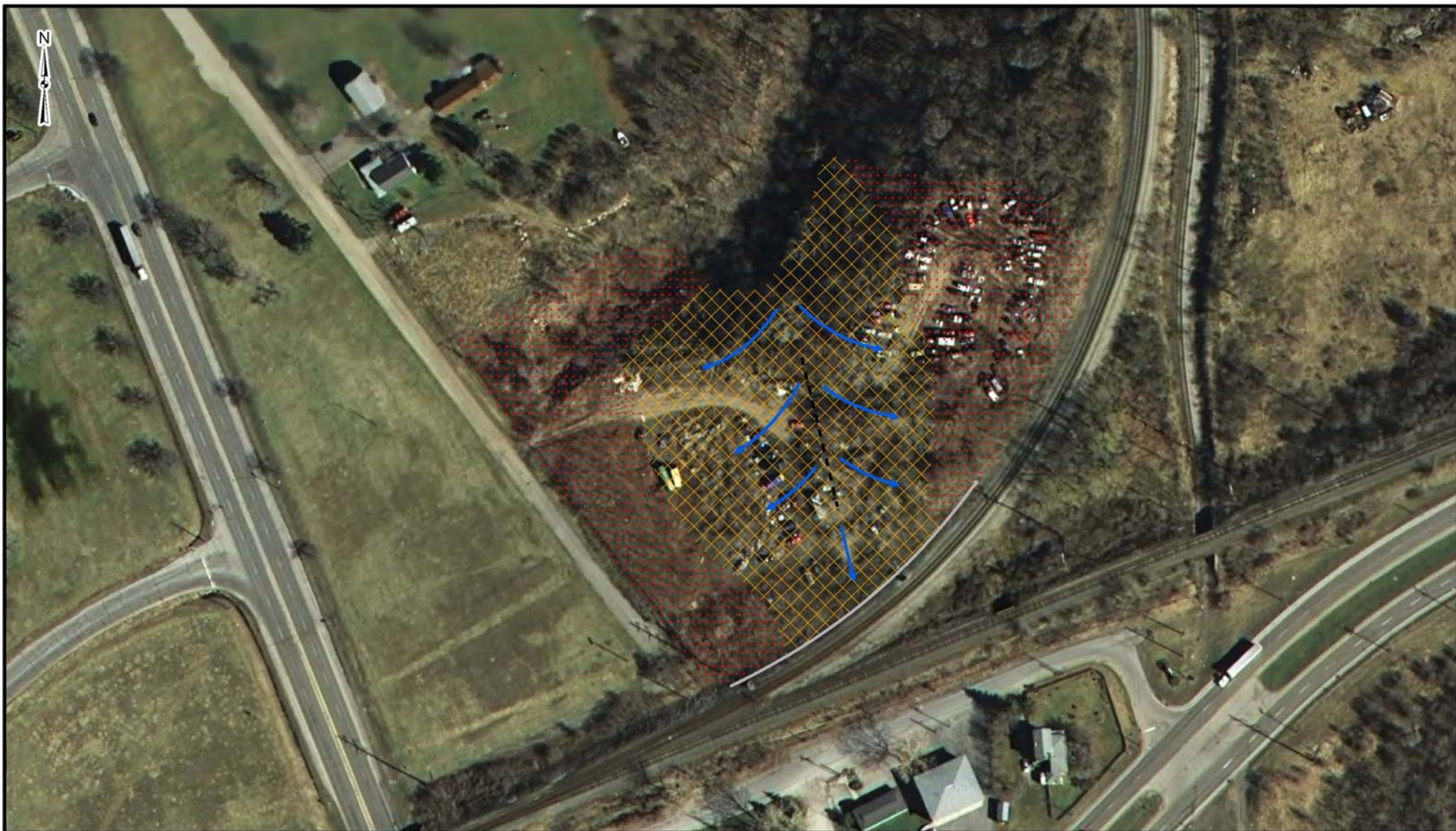
FIGURE 6-6 OU1 Alternative 7: Partial Removal and Off-Site Disposal with In-Situ Stabilization of Shallow Waste
