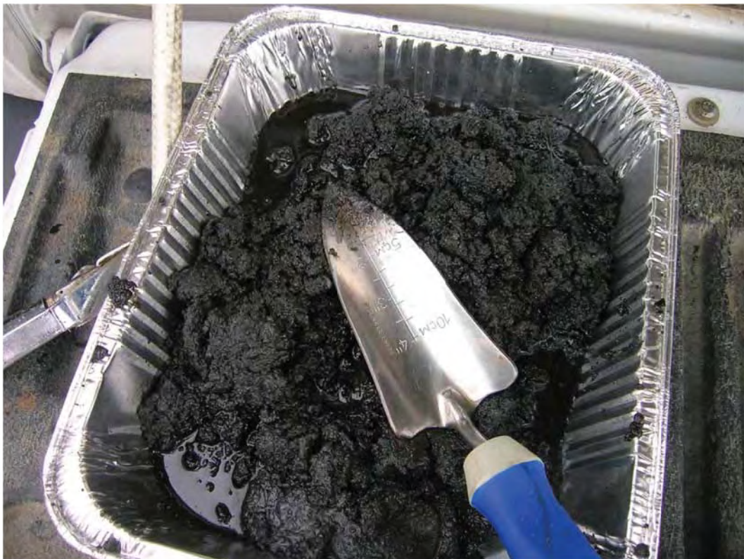
Picture #10- Sediment sample material from Oil Skimmer directly below manhole
