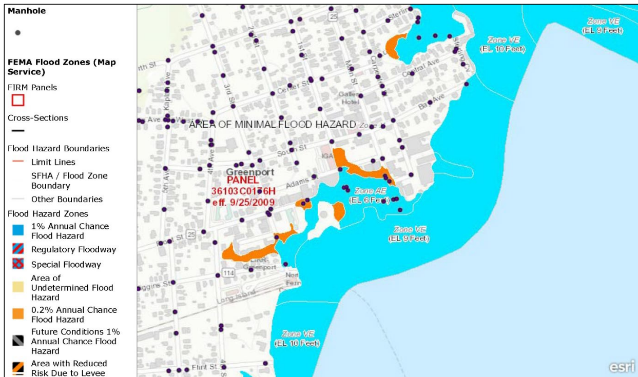
Figure 6. This map shows the location of manholes relative to FEMA Flood Zones.
