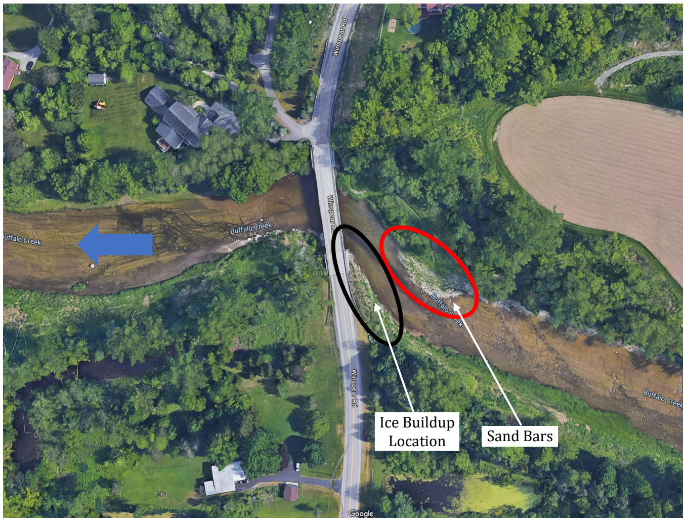
Figure 7. Ice buildup and sand bar locations upstream the Winspear Road bridge in the Town of Elma, NY.
