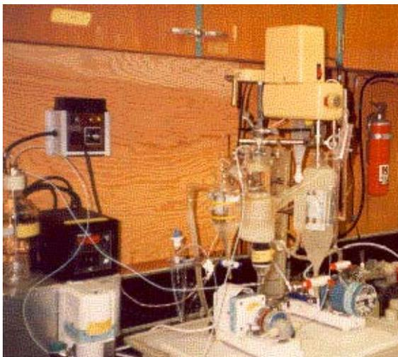
Figure 2. Goulden Large Sample Extractor set up in Environment Canada's monitoring station in Fort, Erie, Ontario.
