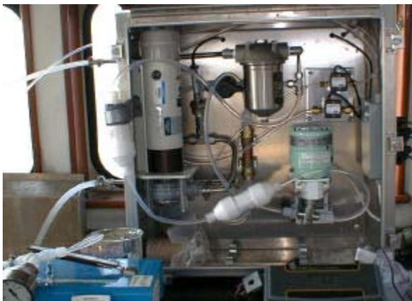
Figure 3. TOPS on the EPA's New York Harbor Survey Vessel *Clean Waters*. The "U" shaped device near the top holds a cartridge filter and the two white double-ended cartridges hold XAD. The two small boxes in the upper right side are flow meters.
