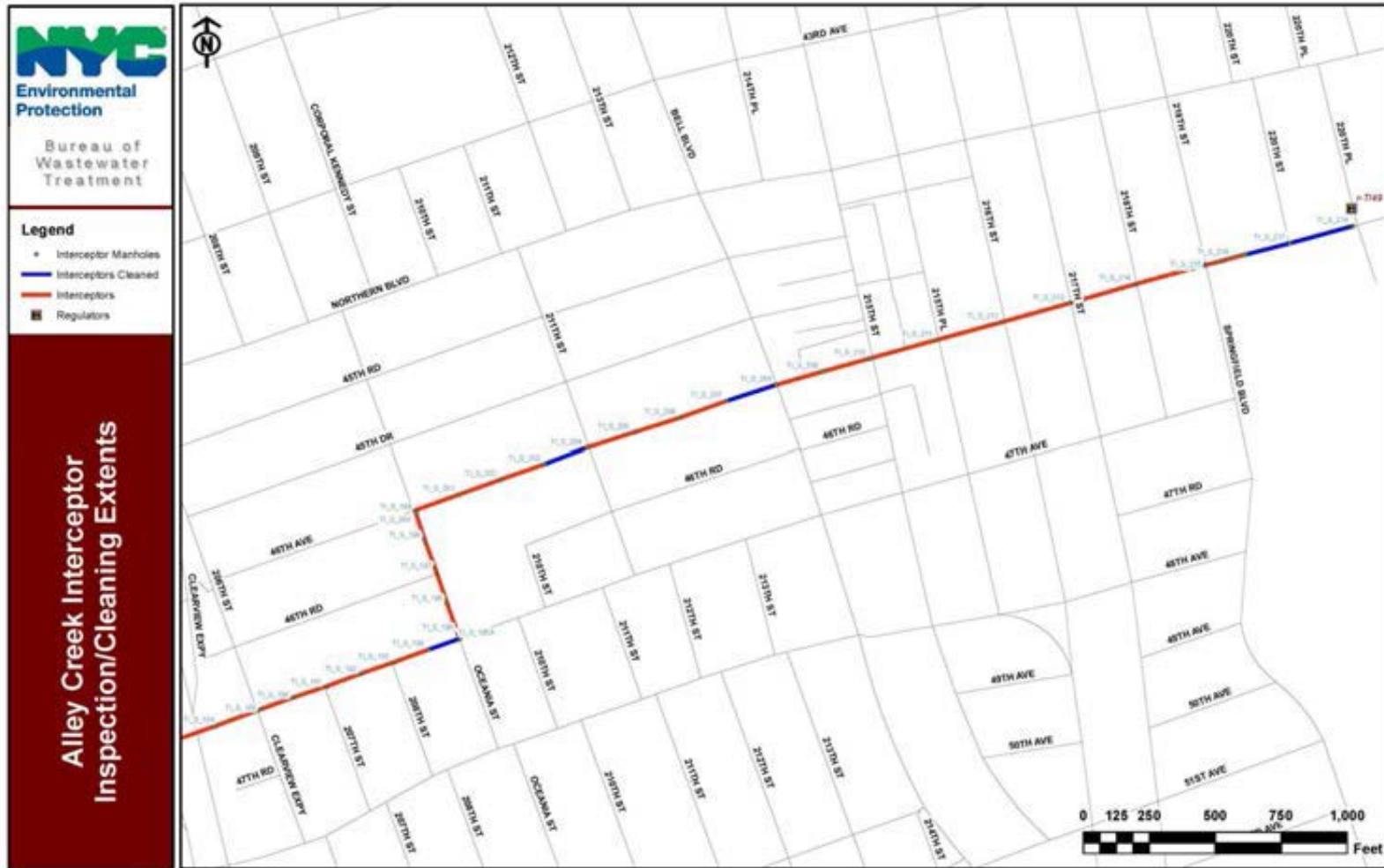
Figure 2-15. Alley Creek Interceptor Inspection Cleaning Extents
