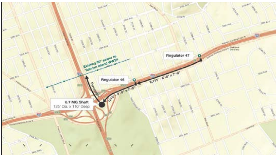
Figure 8-11. Alternative 3B – 6.7 MG Upstream Tank
