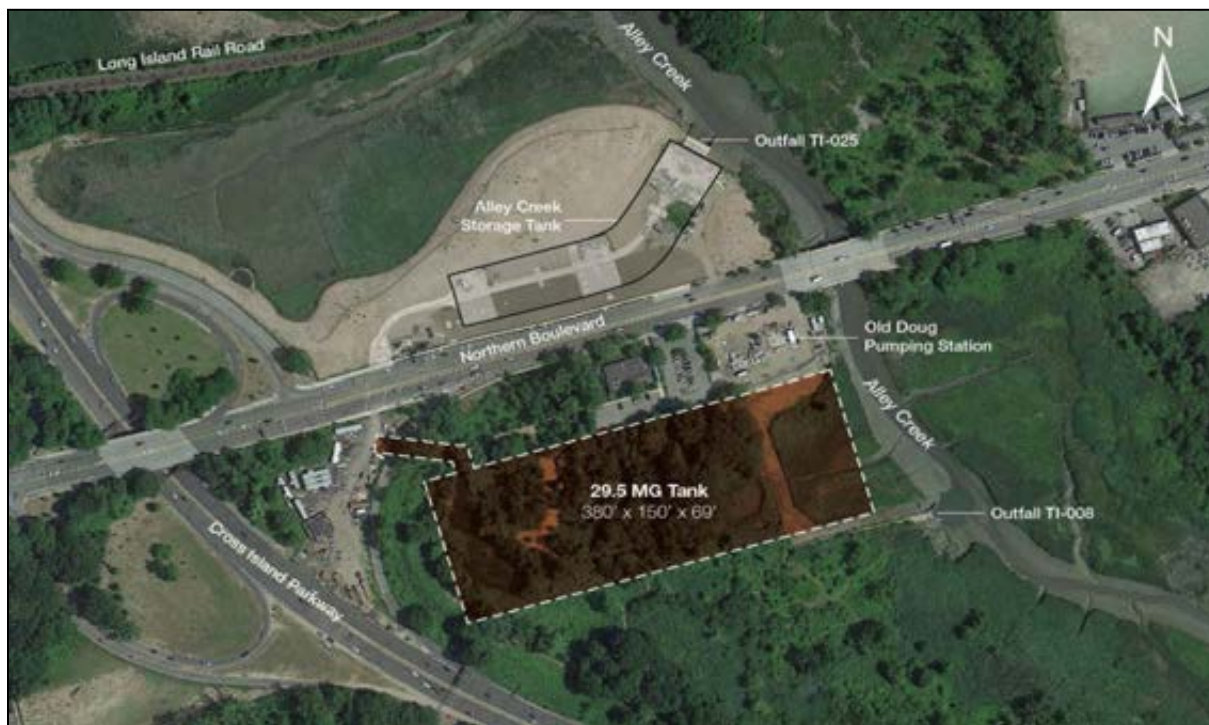
Figure 8-9. Alternative 2D – 29.5 MG Downstream Tank
