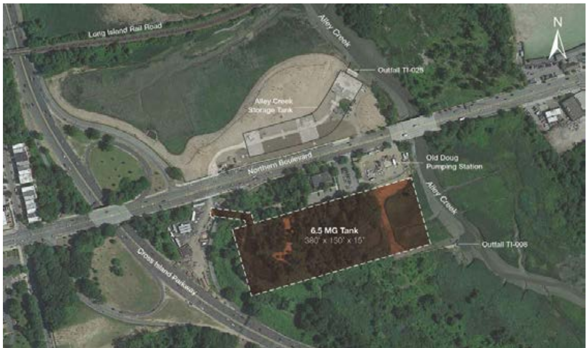
Figure 8-6. Alternative 2B – 6.5 MG Downstream Tank
