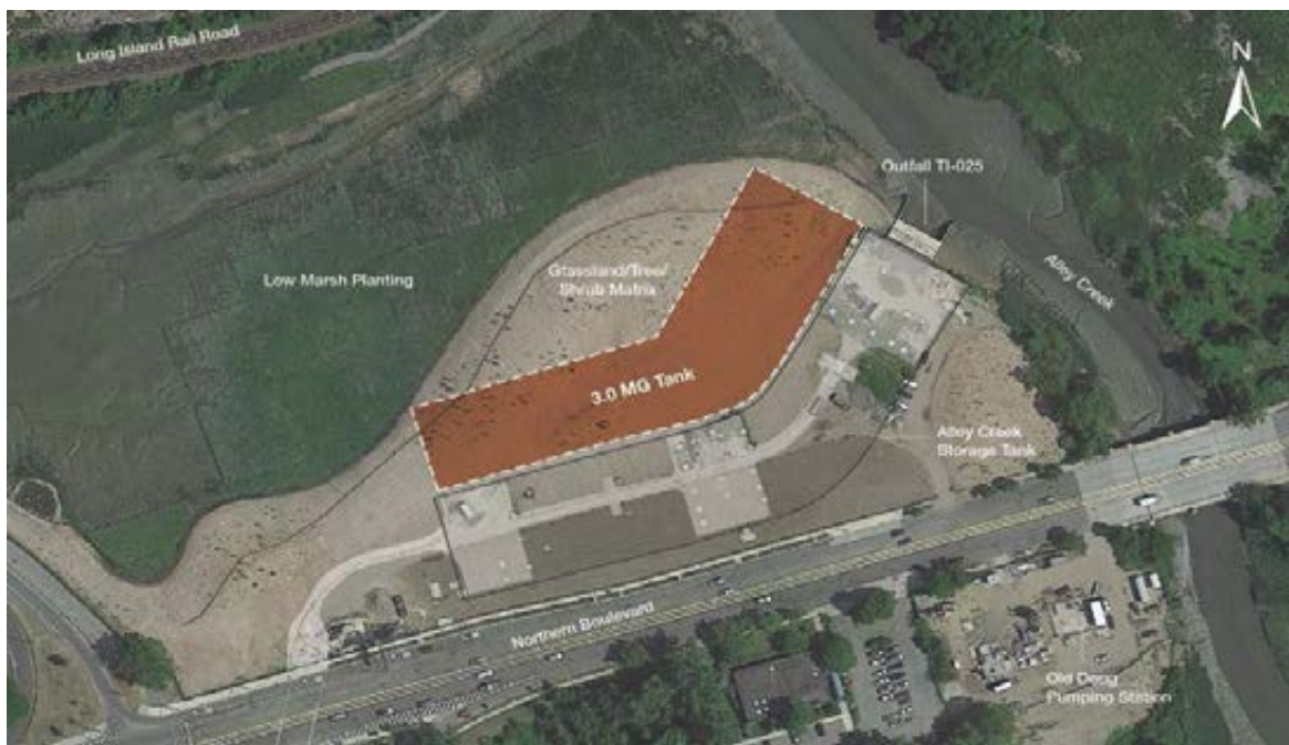
Figure 8-4. Alternative 2A – 3.0 MG Downstream Tank
