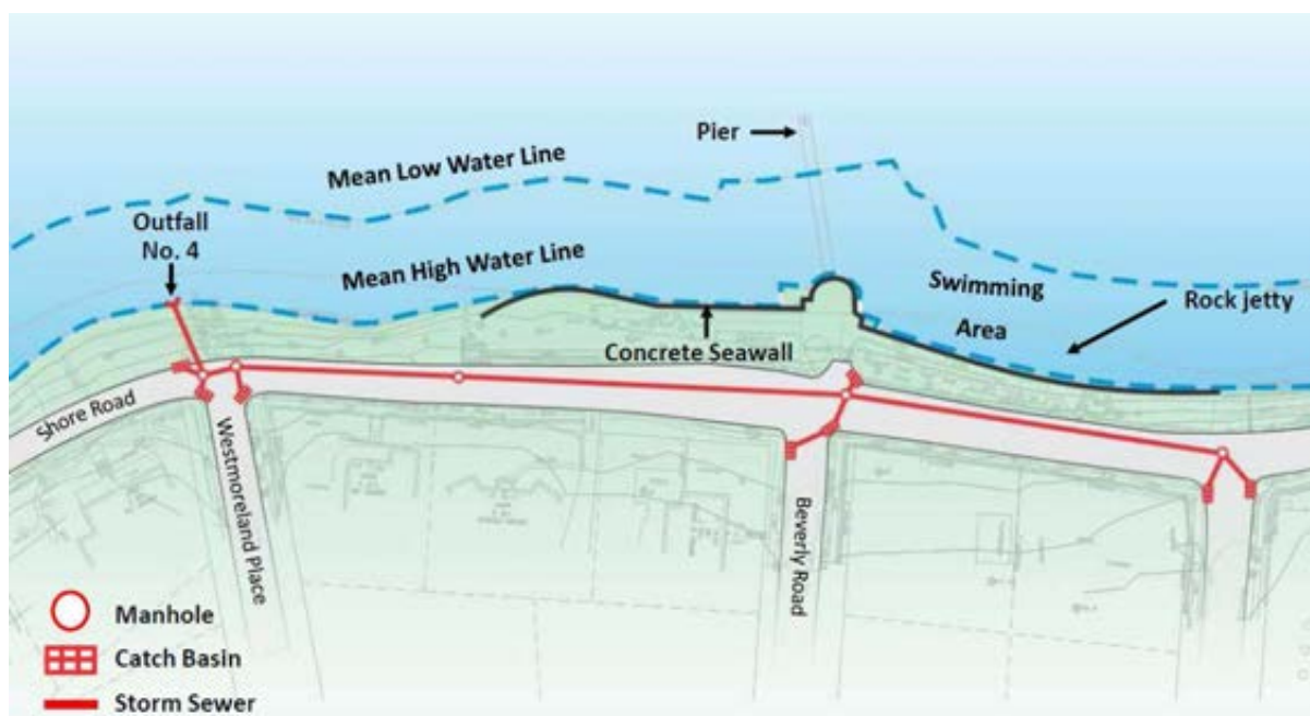
Figure 2-14. DMA Planned Drainage Improvements
