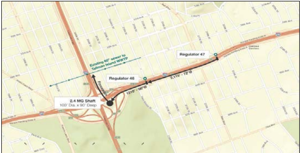
Figure 8-10. Alternative 3A – 2.4 MG Upstream Tank
