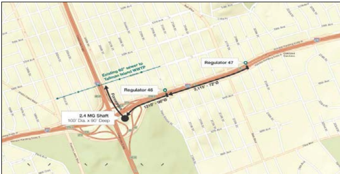
Figure 8-10. Alternative 3A – 2.4 MG Upstream Tank
