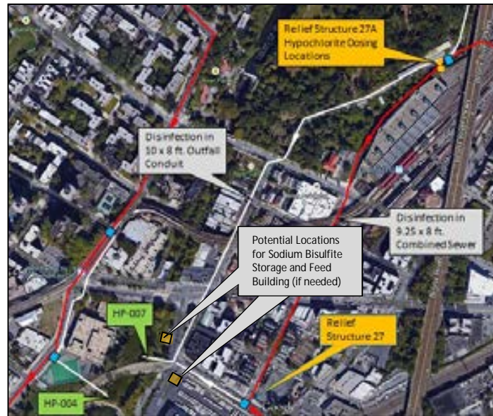
Figure 8-15. Layout of Alternative 7-4 – Outfall HP-007 Direct Disinfection
