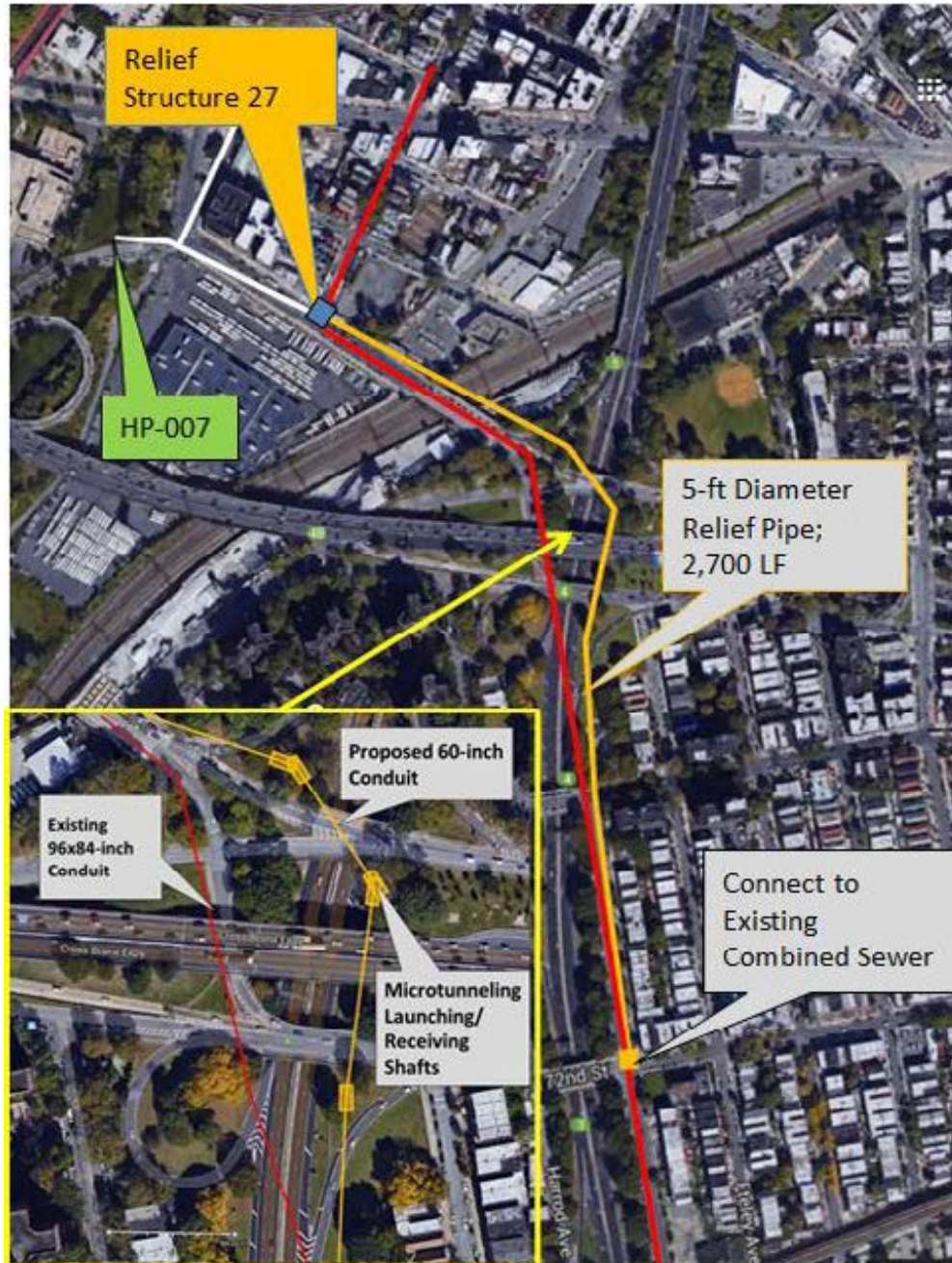
Figure 8-4. Layout of Alternative 7-1 - Hydraulic Relief of CSO Relief 27 at CSO Outfall HP-007
