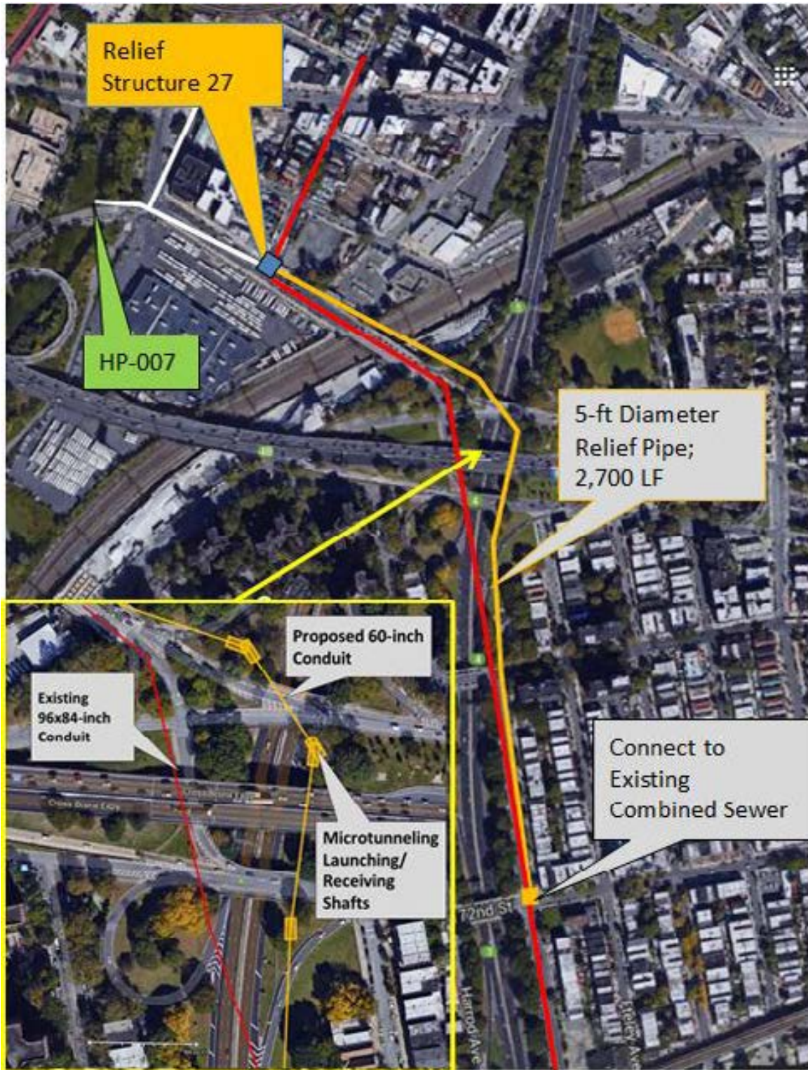
Figure 8-29. Layout of Alternative 7-1 - Hydraulic Relief of CSO Relief 27 at CSO Outfall HP-007
