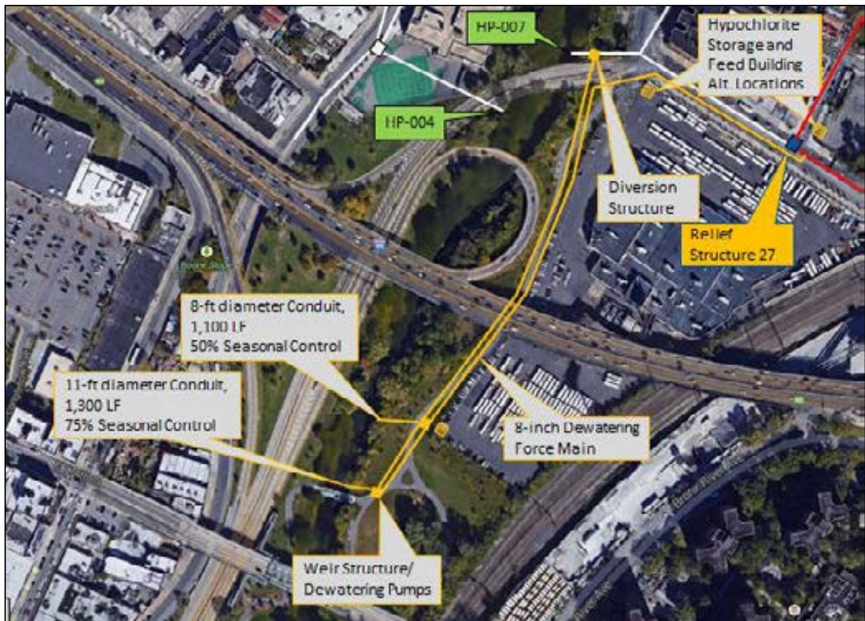
Figure 8-12. Layout of Alternative 7-2 – HP-007 Outfall Conduit Disinfection
