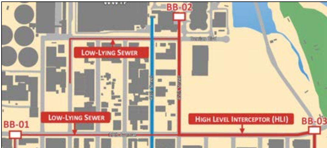
Figure 4-1. Diversion of Low-Lying Sewers near Bowery Bay WWTP into the High Level Interceptor
