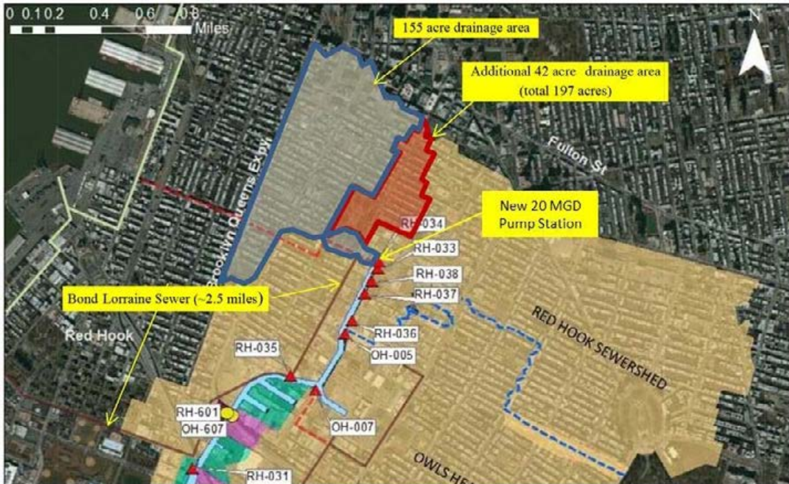
Figure 8-4. Alternatives Layout for Bond Lorraine Sewer
