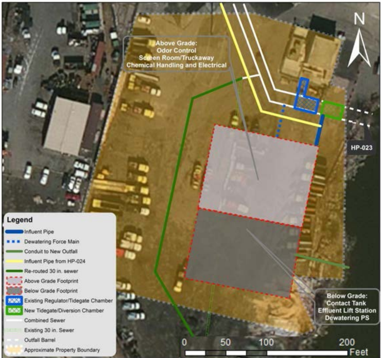
Figure 8-8. Consolidated RTB with Seasonal Disinfection Facility at HP-023
