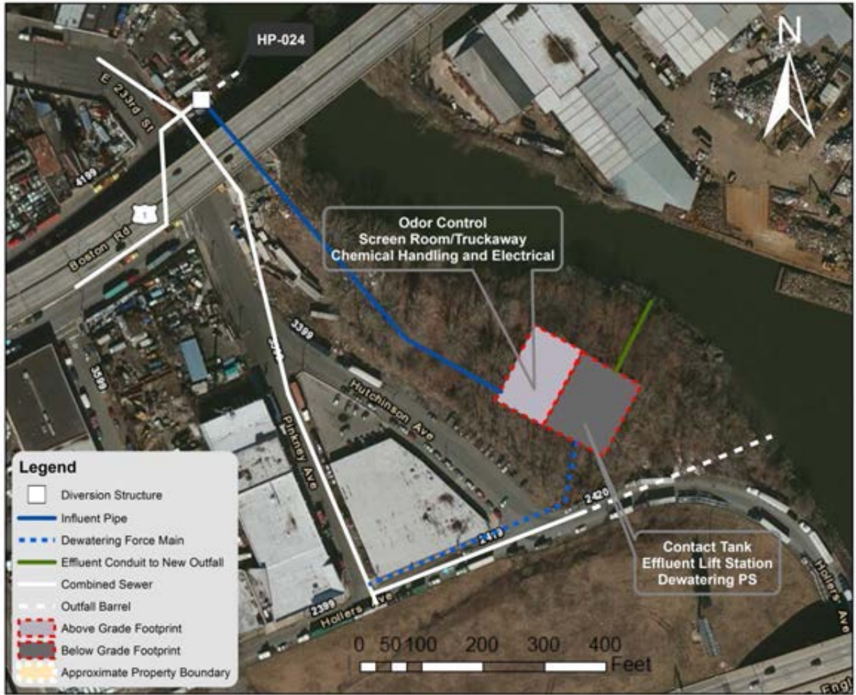
Figure 8-6. RTB with Seasonal Disinfection Facility at HP-024
