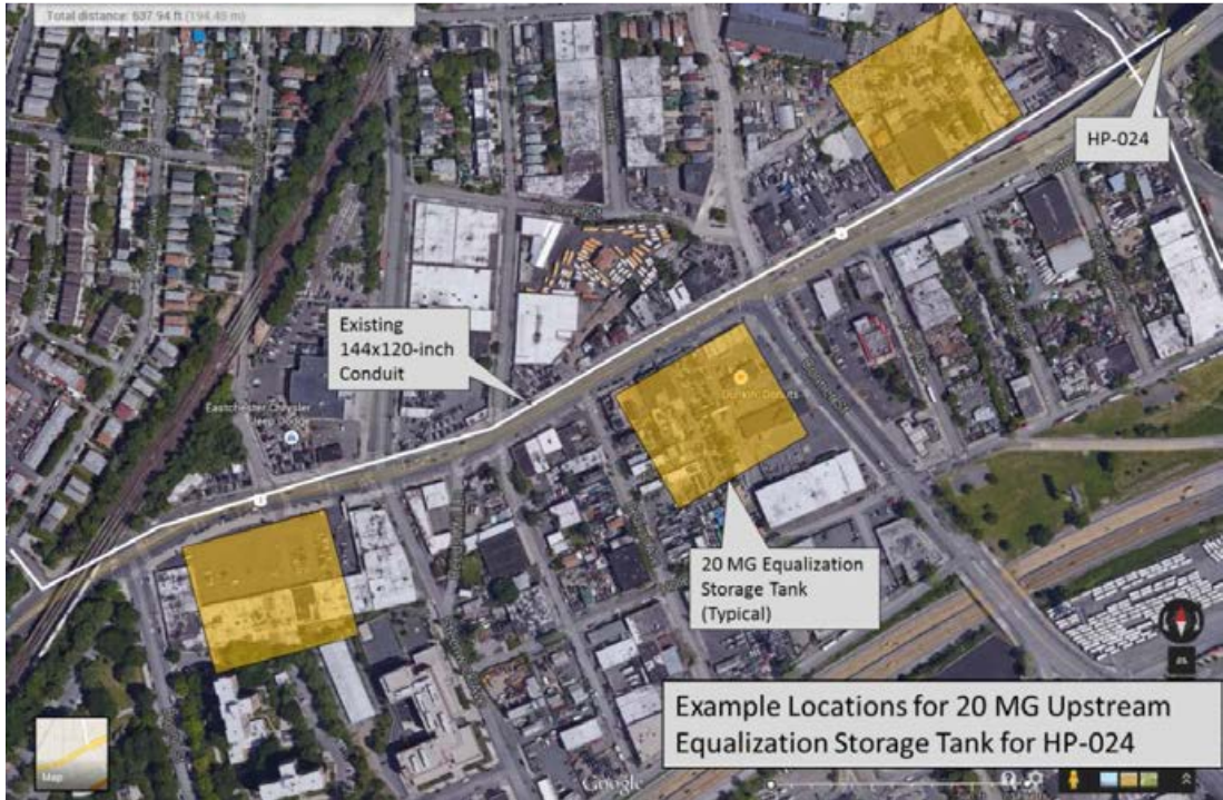
New Figure E-8-3. Siting Options for Upstream Equalization Storage Tank for HP-024- Along Boston Rd.
