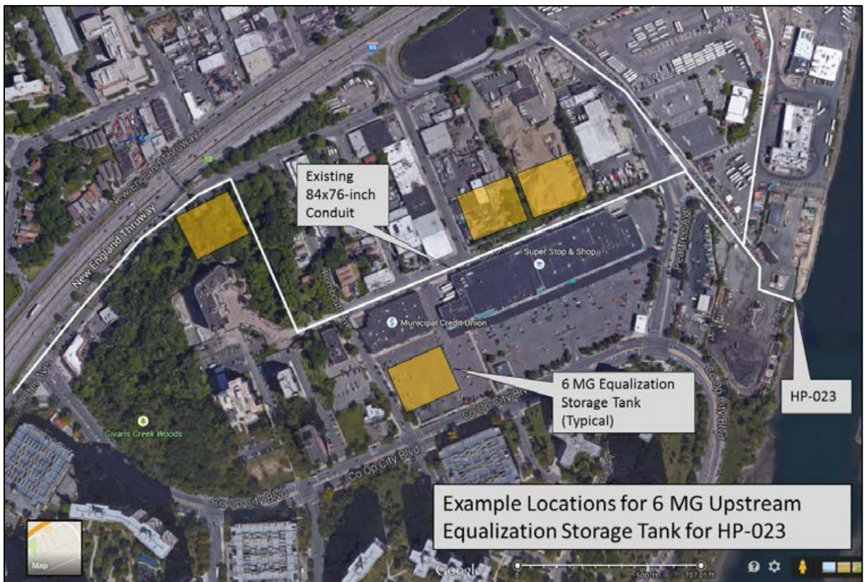
New Figure E-8-4. Siting Options for Upstream Equalization Storage Tank for HP-023
