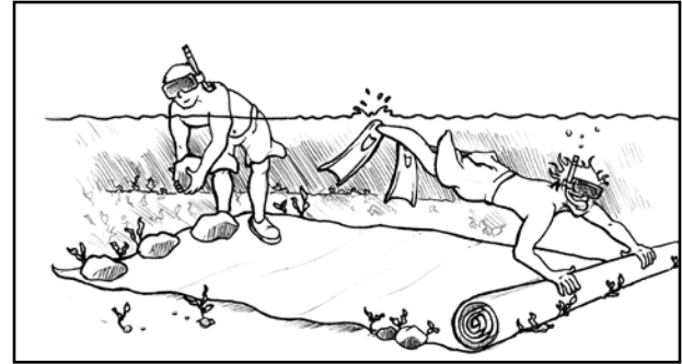
Fig. 6-4. Benthic barriers clear small areas by blocking sunlight and eliminating space where weeds can grow.
