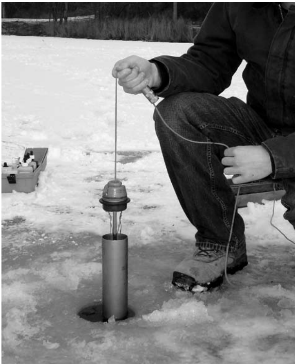
Fig. 5–4. Late-winter water-quality sampling may indicate limiting factors, such as low oxygen levels, that will reduce fish survival and production. The device shown can collect samples at various depths beneath the ice. (CREDIT: JOHN FOSTER)
