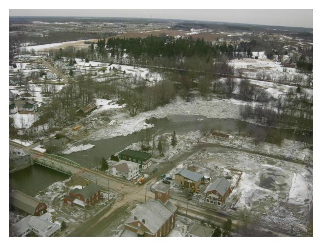
Figure 4-7: Ice buildup in the village of Champlain. Note US-9 bridge at center left is closed, and ice rafts had deposited in developed overbank areas. Orientation is northwest, with flow left to right in image. Image is provided by Clinton County Department of Emergency Services.
