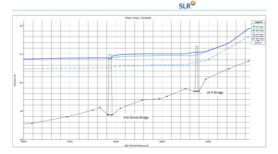
Figure 4-6: Flood Profiles under Existing and Proposed Clear Water Flood Conditions in the Village of Champlain with Lake Champlain at Median April Stage
