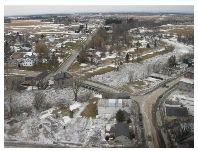
Figure 4-8: Ice jamming in village of Champlain; view is to the east, looking downstream toward Lake Champlain. Elm Street bridge is in center. Breakup ice accumulates at Lake Champlain tailwater ice at center right of image. Image is provided by Clinton County Department of Emergency Services.
