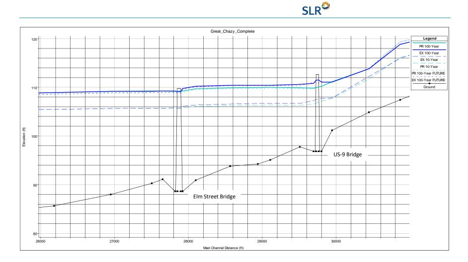
Figure 4-5: Flood Profiles under Existing and Proposed Clear Water Flood Conditions in the Village of Champlain with Lake Champlain at Corresponding Flood Stages
