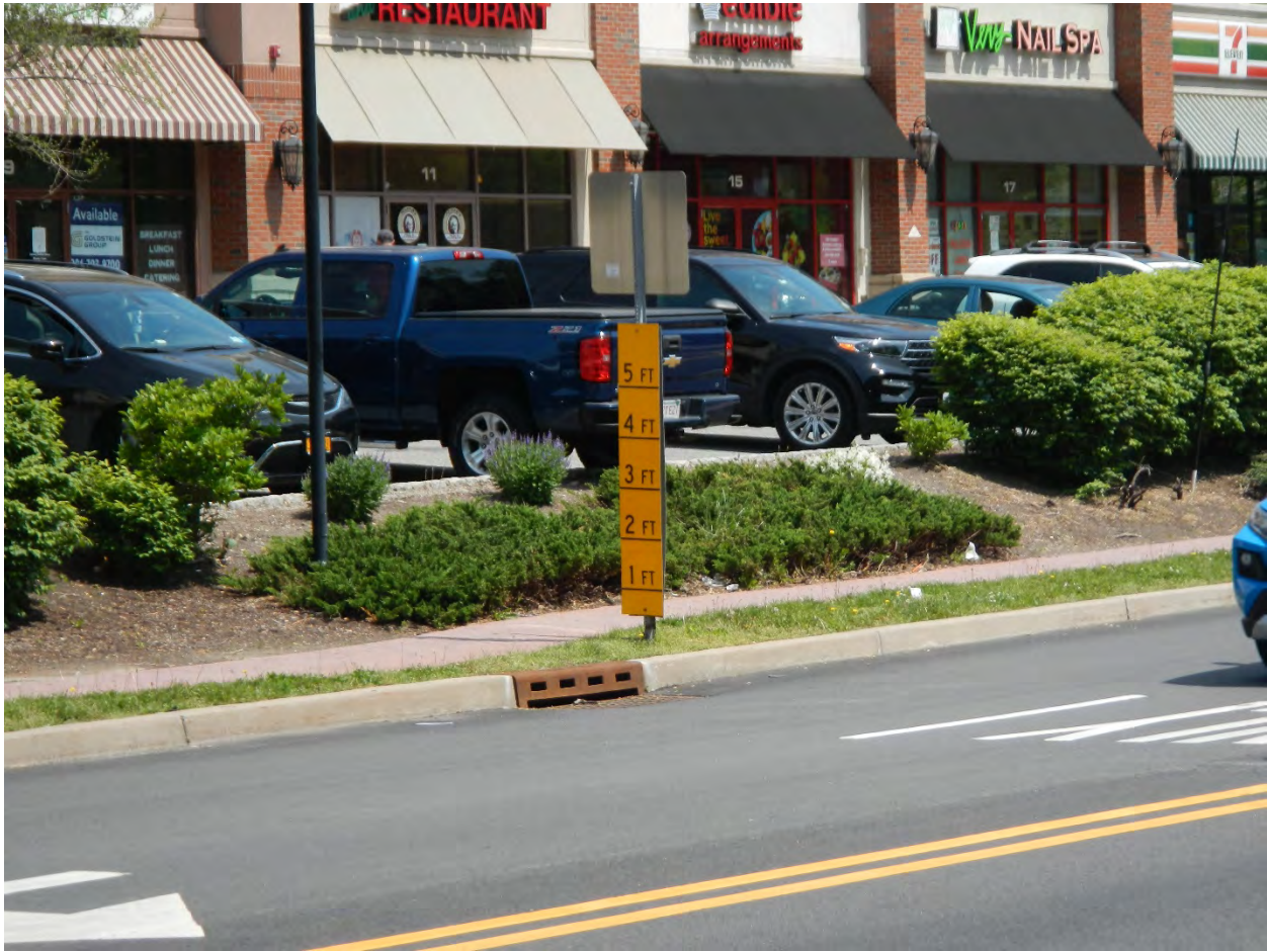
Figure 4-8: Flood stage indicator on the north side of the Franklin Turnpike on Mahwah River's right overbank. In the 100-year flood, depths of nearly 7 feet are modeled at this location under existing conditions.
