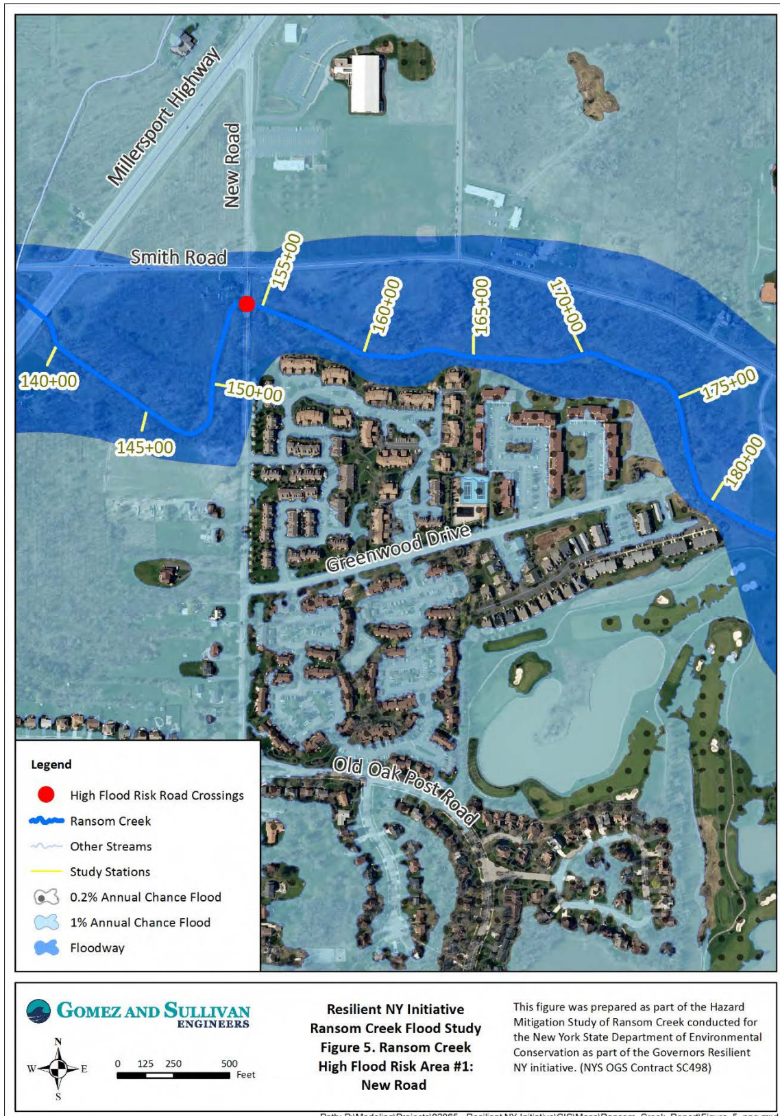
Figure 5. Ransom Creek High Flood Risk Area #1: New Road
