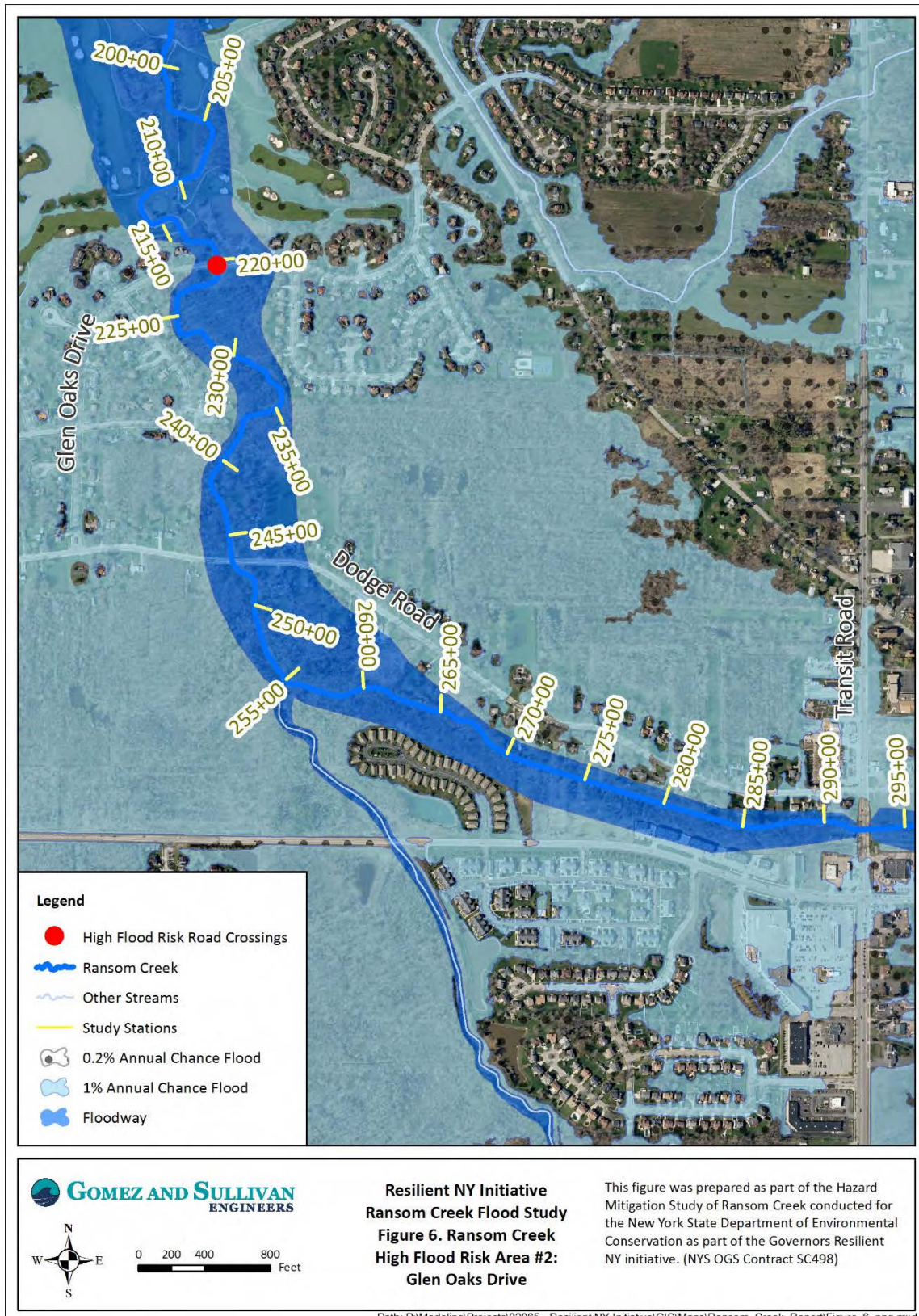
Figure 6. Ransom Creek High Flood Risk Area #2: Glen Oaks Drive
