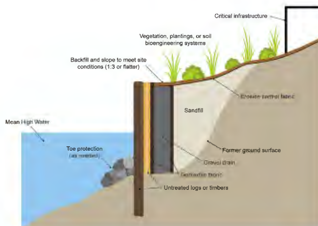
FIGURE 12: Typical detail, timber bulkhead
