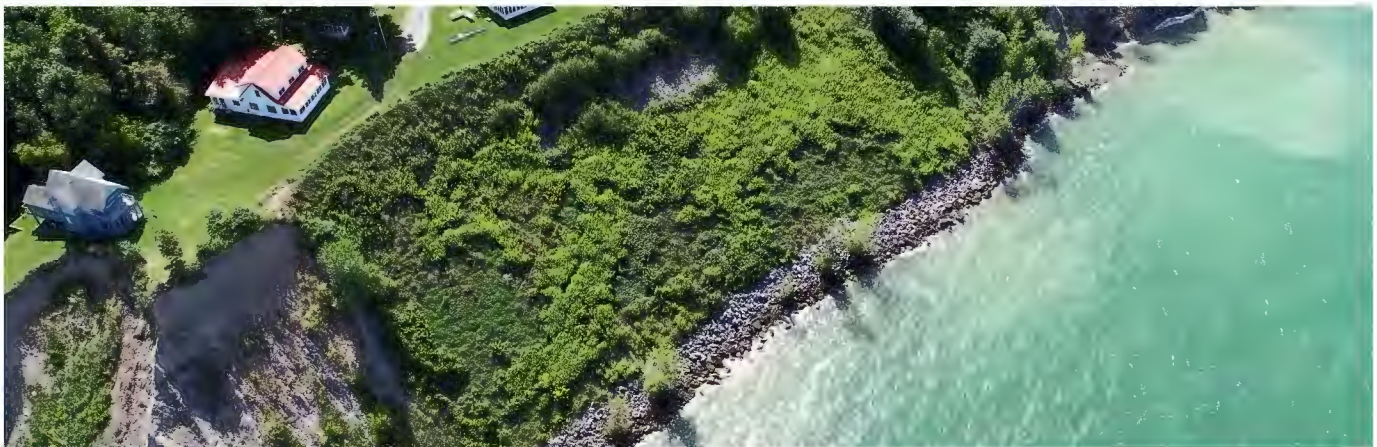
PHOTO 13. Re-graded slope with toe protection and vegetative planting near Sodus Bay
