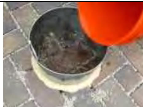
Infiltration test using ASTM C-1701
