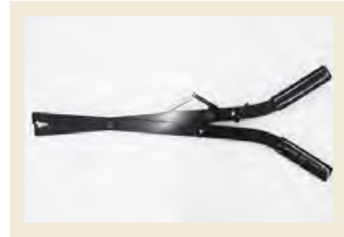
Figure 26. Selflocking bodygrip trap setter
