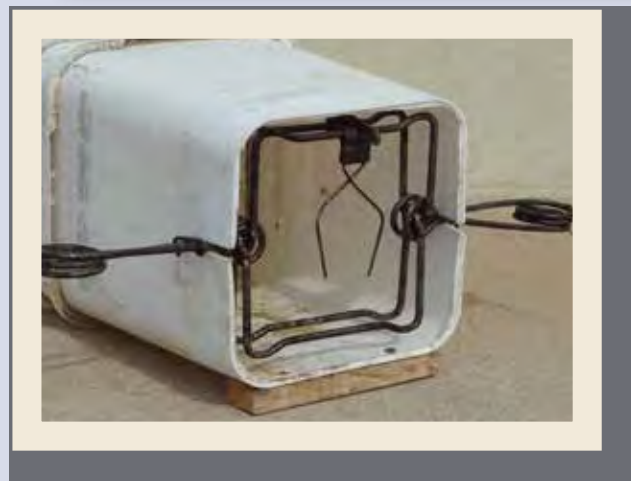
Figure 4. Typical trigger configurations; placement is top center and shape is inverted "U" or "V."
