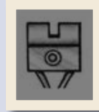
Figure 1B. Square notch non-adjustable tension (riveted) trigger; 1 or 2 way
