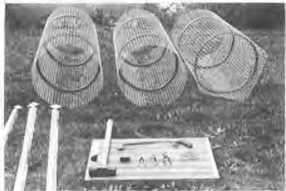
FIGURE 2. MATERIALS AND TOOLS FOR CONSTRUCTING A POND LEVELER
