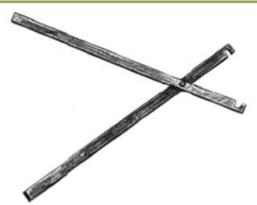
Figure SK3. Setting tool
