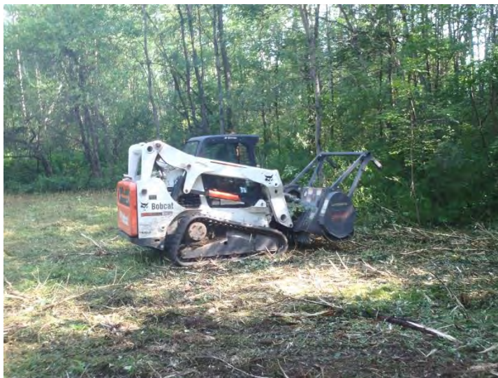
Photo 2: Shrubland management using a forestry mower.
