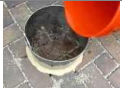
Infiltration test using ASTM C-1701
