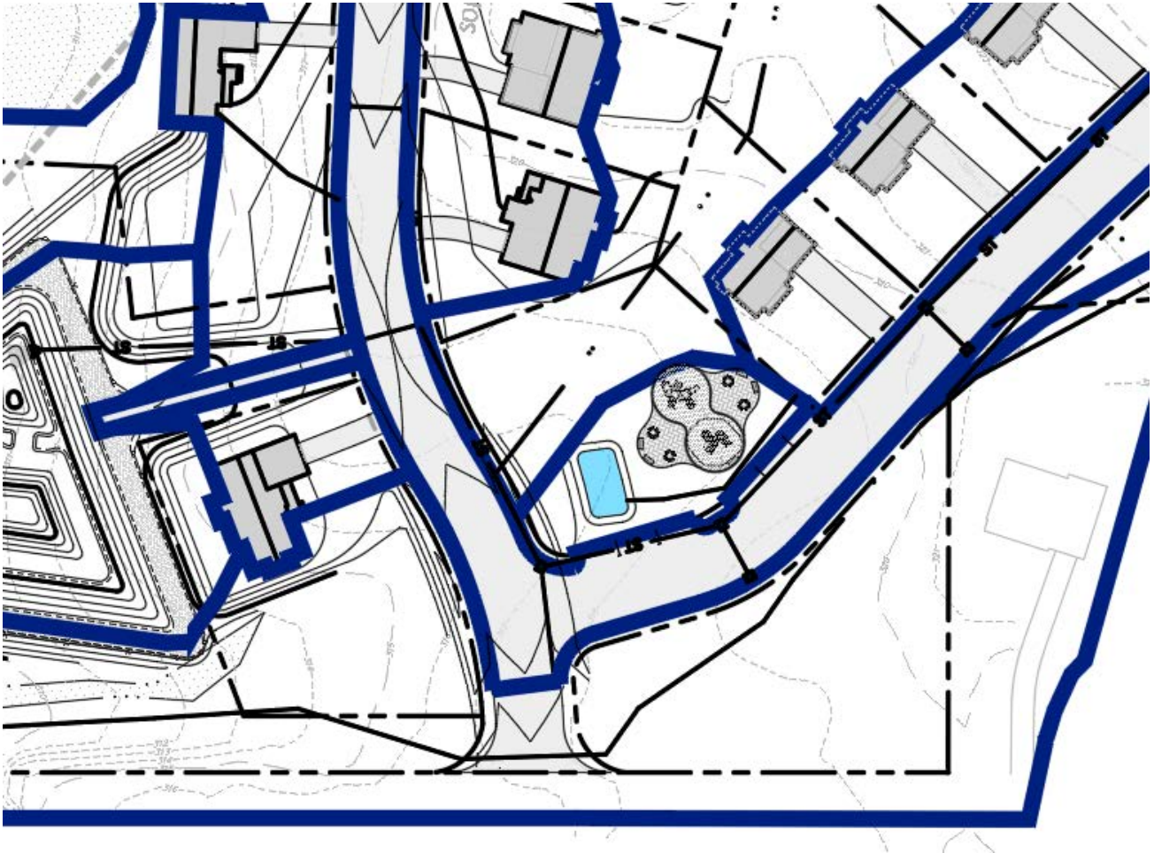
Figure 7.15 Post-development Filtration Bioretention Area
