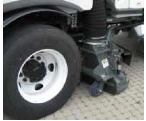
Routine, air-vacuum sweeping in the early spring and fall is the best approach for porous pavement maintenance (Photo source: Toronto and Region Conservation)
