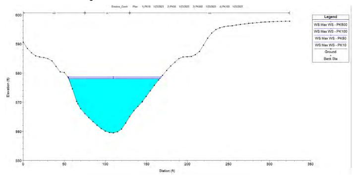
Figure 4 Water Surface elevations for Cross Section 880
