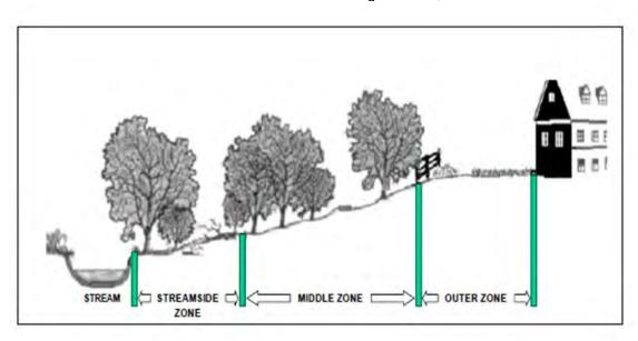
Figure 1 – Three-Zone Stream Buffer DEC Stormwater Design Manual, 2015
