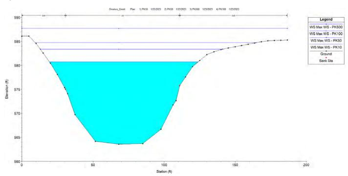
Figure 5 Water Surface Elevation for Cross Section 5742
