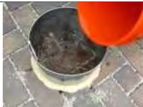
Infiltration test using ASTM C-1781
