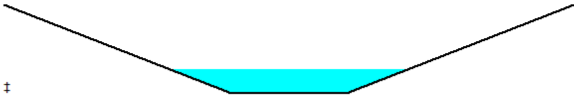
Figure 7.23 2-Year Flow Depth in Dry Swale
