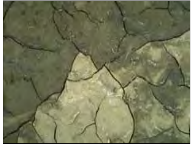
Figure 5.15 Shows typical compacted soils that nearly reach the bulk density of concrete (Schueler et al 2000)
