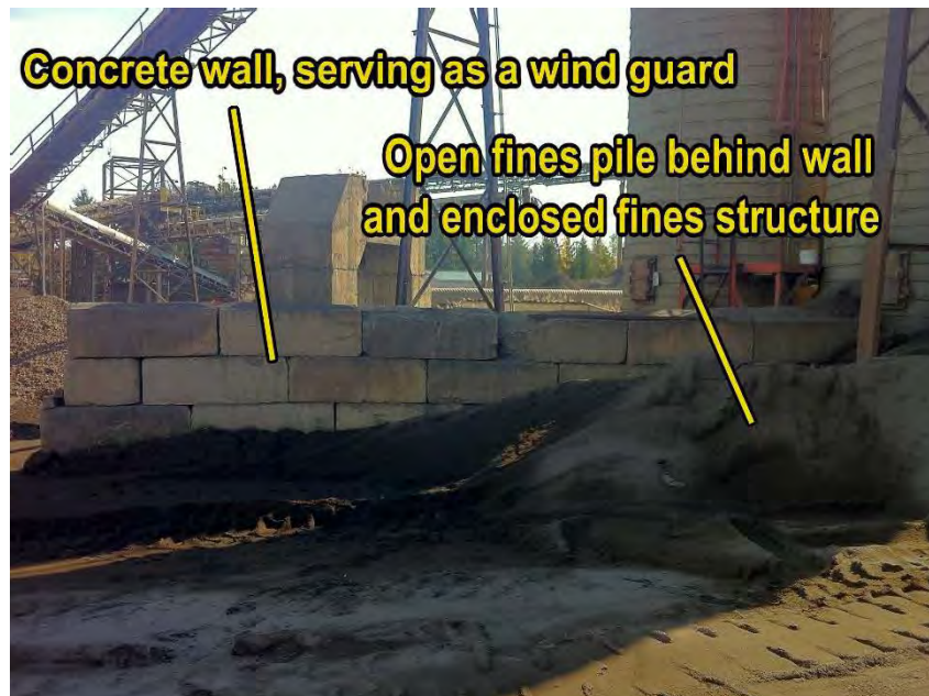
Photo 4. Open fines area, showing concrete wall on eastern side of pile which acts as a barrier against wind erosion.
