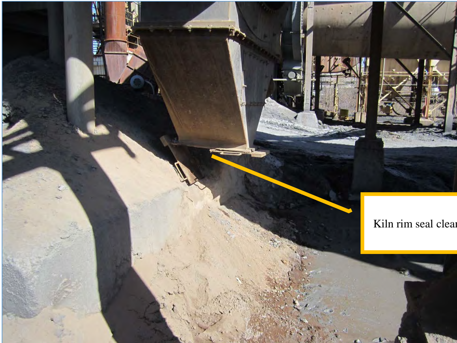
Kiln Feed Area Photograph 10, looking west: The kiln rim seal chute is opened (KF31) for cleaning.
