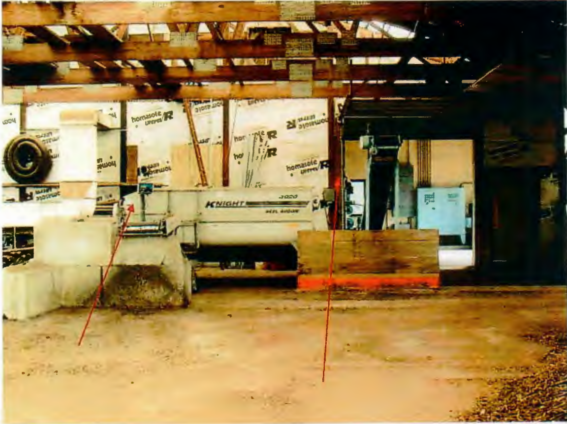
Note: Scale on mixer (left hand side) .....press discharge on right. Biosolids sampling here.
