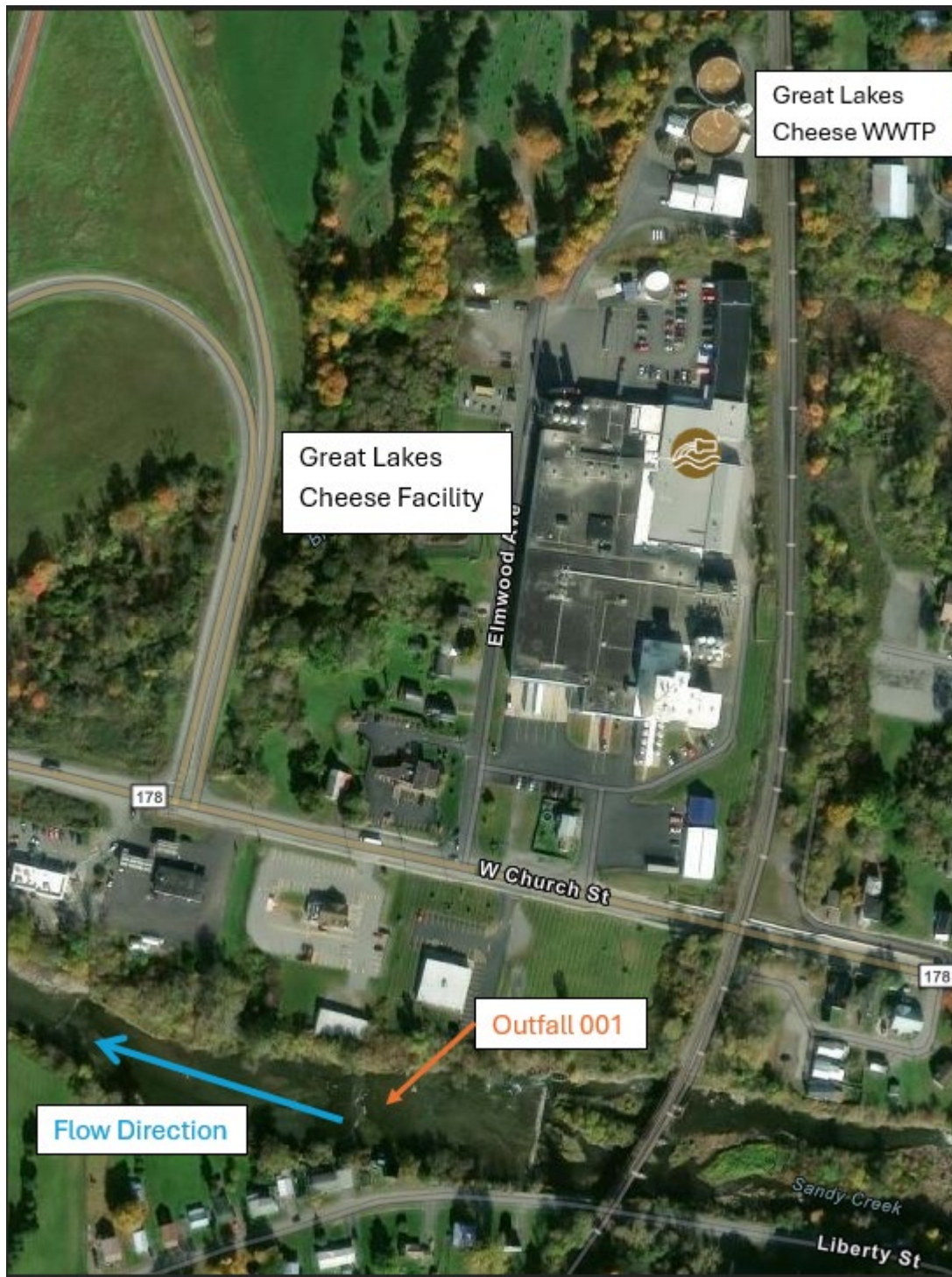
Figure 2. Overhead view of the Great Lakes Cheese facility, including the process facility, wastewater treatment plant, and approximate location of Outfall 001 in Sandy Creek (WIN: ONT-44 portion as described).
